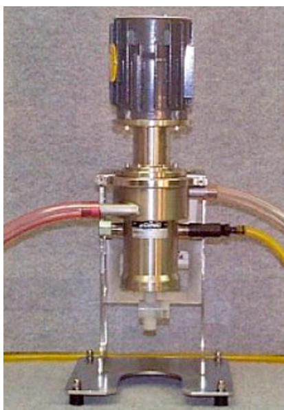
**Figure 3.** Laboratory scale extraction centrifuge (courtesy of CINC Inc.).
