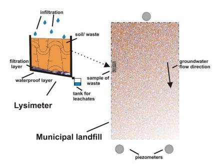
Figure 1. General sketch of the lysimeter.
