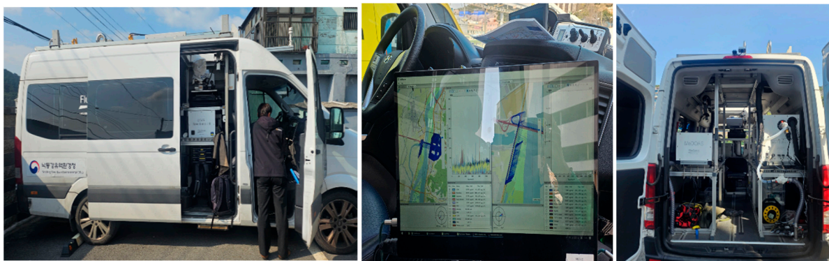
Figure 2. Me-DOAS measurement system mounted on the SOF (solar occultation flux) vehicle.
