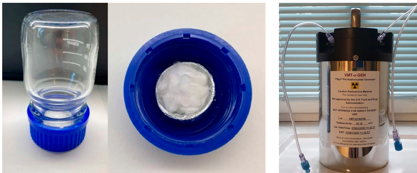
Figure 1. Prototype ^{224}\text{Ra}/^{212}\text{Pb} generator from CERN (duran-flask-emanation-based) and the wet-chemical-based ^{224}\text{Ra}/^{212}\text{Pb} generator (VMT- \alpha -GEN) from Perspective Therapeutics.
