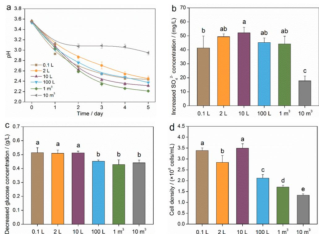
**Figure 2.** Properties of microbial solutions during the scale-up cultivation process of mixotrophic acidophiles. (a) Solution pH. (b) Increased sulfate radical concentration. (c) Decreased glucose concentration. (d) Cell density. Different small letters indicate significant ( $p < 0.05$ ) differences according to the LSD test.
