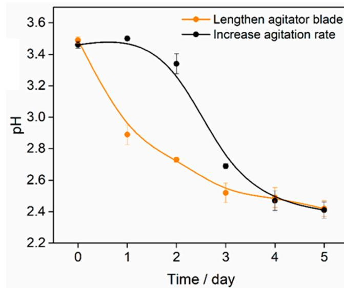
**Figure 7.** Solution pH changes in the cultivation system of 10 m<sup>3</sup> after modifying the bioreactor parameters. Red and black lines represent the modifications of lengthening the agitator blade and increasing the agitation rate.
