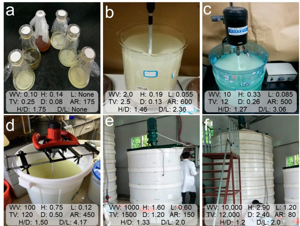
**Figure 1.** Bioreactor parameters used for the scale-up cultivation process of mixotrophic acidophiles. (a–f) Scale-up cultivation stages of 0.1 L, 2 L, 10 L, 100 L, 1 m<sup>3</sup>, and 10 m<sup>3</sup>, respectively. WV, work volume (L); TV, total volume (L); H, bioreactor height (m); D, bioreactor diameter (m); L, paddle length (m); AR, agitator agitation rate (rpm).
