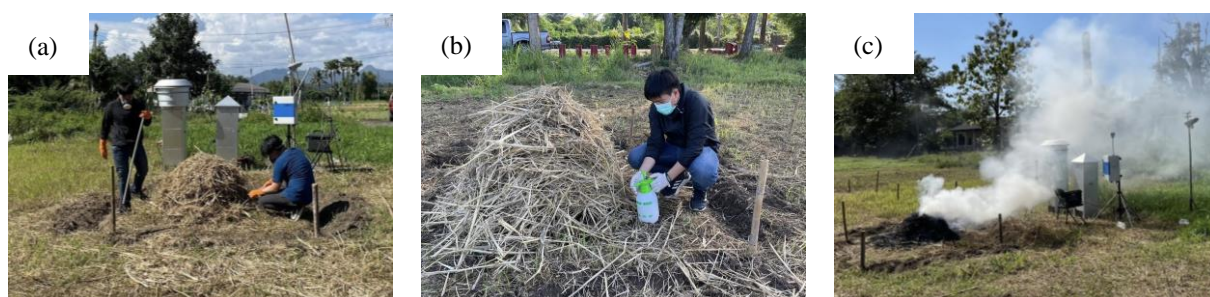
Figure 1. The procedure of open burning process: (a) biomass preparation, (b) pesticide spraying onto biomass, and (c) incomplete combustion and air sampling.
