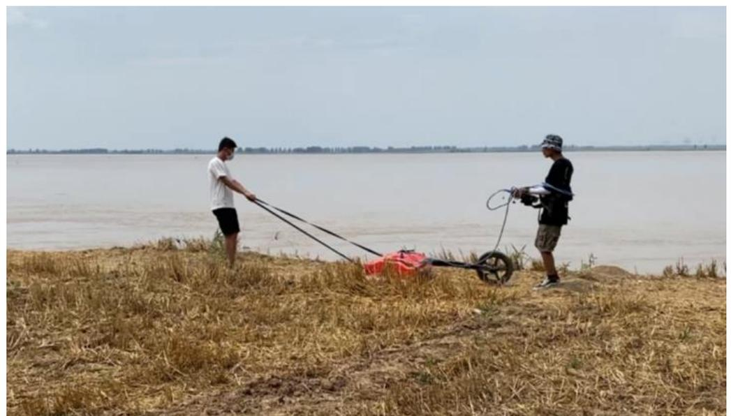
**Figure A1.** Scanning the floodplain in Wantan Town using the geological radar.
