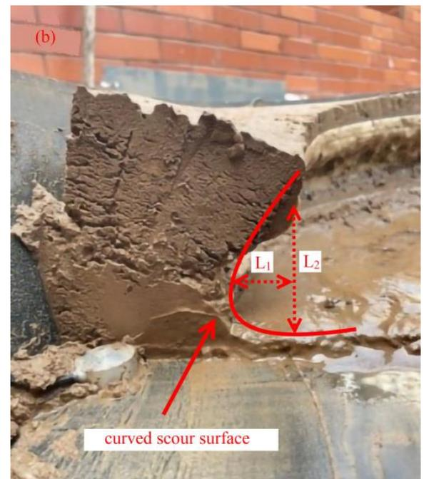
**Figure 6.** Bank failure pattern: (a) failure schematic diagram of slopes under working condition 2; (b) actual diagram of the concave bank under working condition 2 (L<sub>1</sub>: the scour height, L<sub>2</sub>: the scour width).
