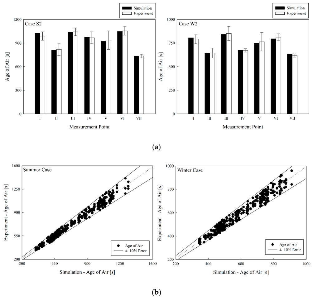
**Figure 5.** Comparison of age of air between experiment and simulation; (a) comparison of Cases S2 and W2; (b) comparison of all cases in summer and winter.
