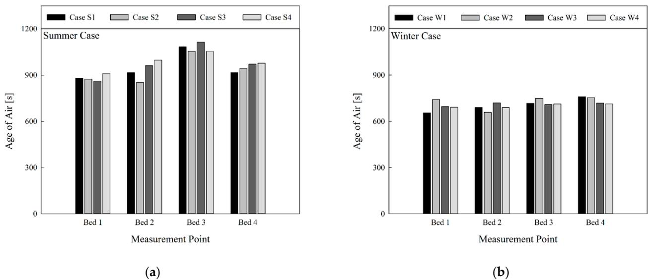
**Figure 6.** Comparison of age of air at bed location by season (in cases of ventilation system operation, four-way cassette fan coil unit operation, non-operation of air cleaner, no use of curtain): (a) summer; (b) winter.
