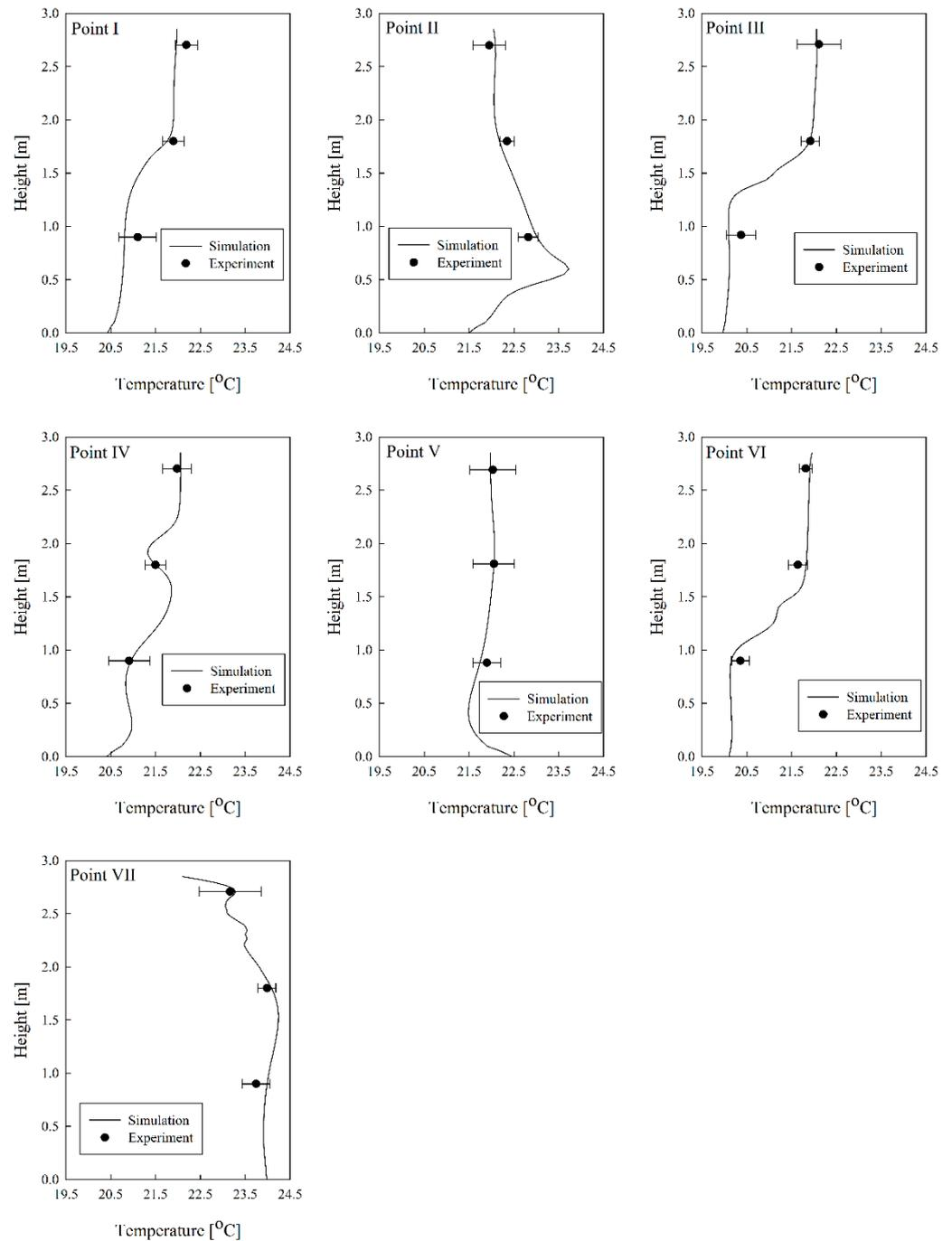
**Figure 4.** Comparison of experimental and simulation results for temperature distribution by height at seven locations in laboratory.
