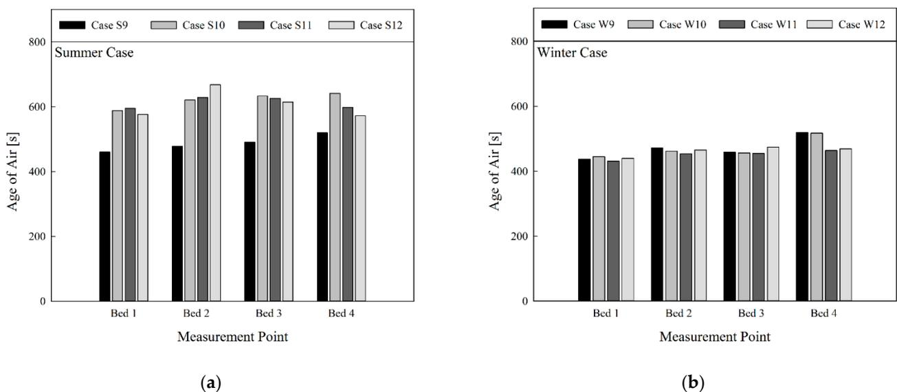
**Figure 8.** Comparison of age of air at bed location by season (in cases of ventilation system operation, four-way cassette fan coil unit operation, operation of air cleaner, and no use of curtain): (a) summer; (b) winter.
