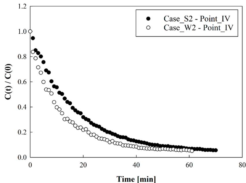
**Figure 2.** One of the measurement results for particle number concentration over time.
