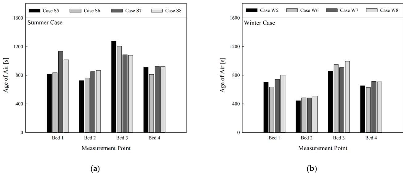
**Figure 7.** Comparison of age of air at bed location by season (in cases of ventilation system operation, four-way cassette fan coil unit operation, non-operation of air cleaner, and use of curtain): (a) summer; (b) winter.
