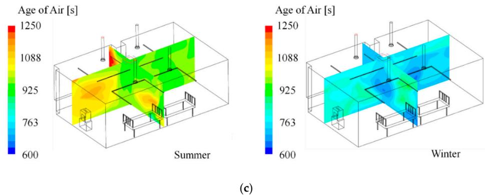
**Figure 3.** One of the simulation results (**left**: Case S2 in summer, **right**: Case W2 in winter); (a) velocity contour; (b) temperature contour; (c) age of air contour.
