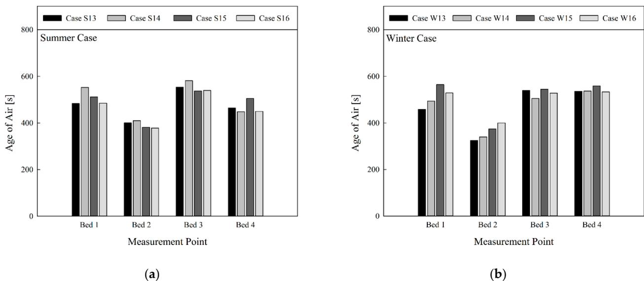
**Figure 9.** Comparison of age of air at bed location by season (in cases of ventilation system operation, four-way cassette fan coil unit operation, operation of air cleaner, and use of curtain): (a) summer; (b) winter.
