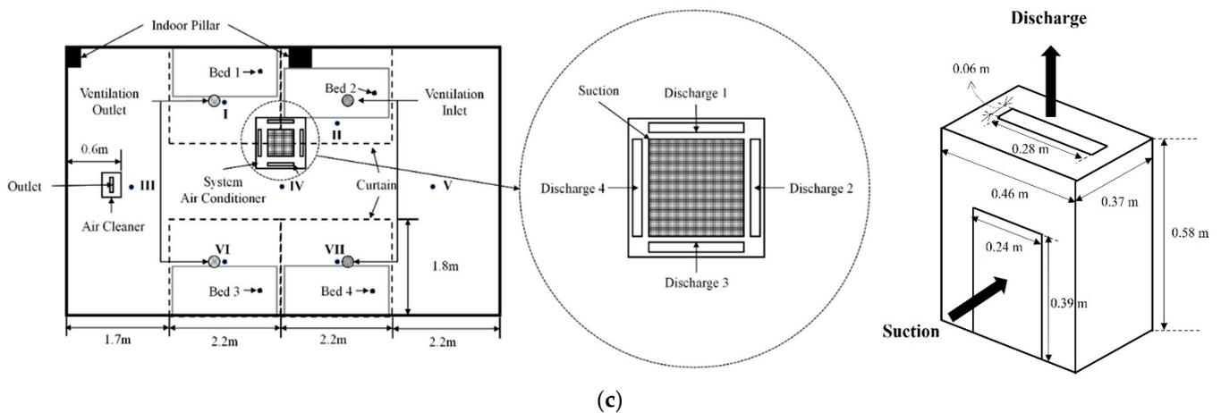
**Figure 1.** Composition of the four-bed ward laboratory: (a) laboratory photograph; (b) isometric view; (c) floor plan.
