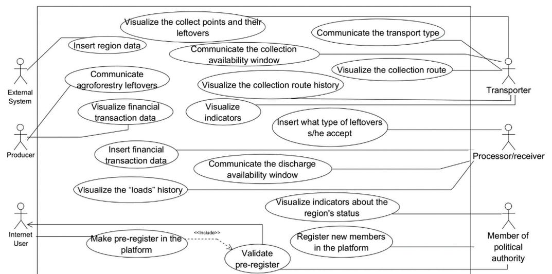
**Figure 2.** Key high-level features of the platform based in use-case diagram from UML.
