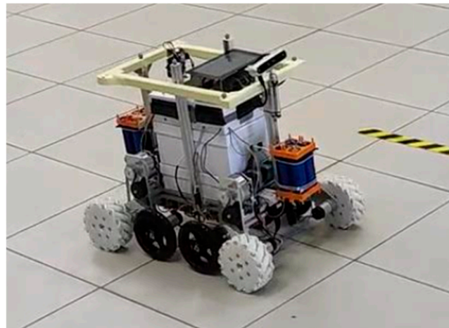
Figure 1. Autonomous mobile robot with differential rotation and dual mounting rails for the RFID system. Source: Personal contribution.
