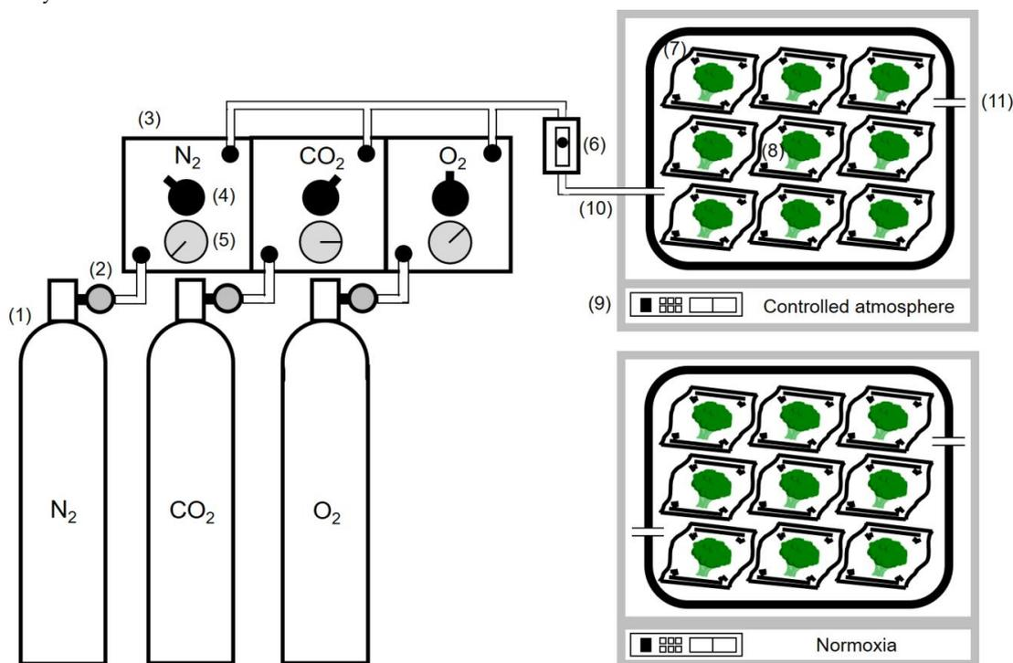
**Figure 1.** Schematic diagram of storage system for broccoli heads under controlled atmosphere and normoxia. (1) Gas cylinders, (2) regulators, (3) LogMIX gas mixture device (Fronto Co., Ltd., Kunitachi, Japan), (4) gas flow controller, (5) pressure gauge, (6) flowmeter, (7) 7-L acrylic jar (V-7, Shin-ei Sangyou Co., Ltd., Daito, Japan), (8) samples (broccoli heads), (9) temperature control units, (10) inlet, (11) outlet.
