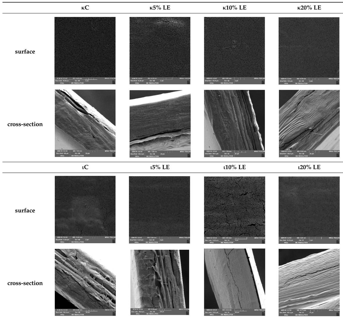
$\kappa$ C— $\kappa$ -carrageenan control film,  $\kappa$ 5% LE— $\kappa$ -carrageenan with 5% of lapacho extract,  $\kappa$ 10% LE— $\kappa$ -carrageenan with 10% of lapacho extract,  $\kappa$ 20% LE— $\kappa$ -carrageenan with 20% of lapacho extract,  $\iota$ C— $\iota$ -carrageenan control film,  $\iota$ 5% LE— $\iota$ -carrageenan with 5% of lapacho extract,  $\iota$ 10% LE— $\iota$ -carrageenan with 10% of lapacho extract,  $\iota$ 20% LE— $\iota$ -carrageenan with 20% of lapacho extract.
