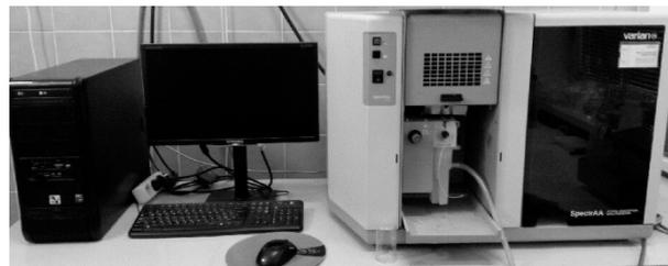
Figure 1. Atomic absorption spectroscopy Varian AA280Z.
