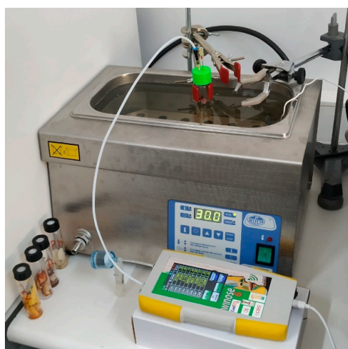
Figure 5. Test of mushrooms with the electronic nose WINOSE 6.
