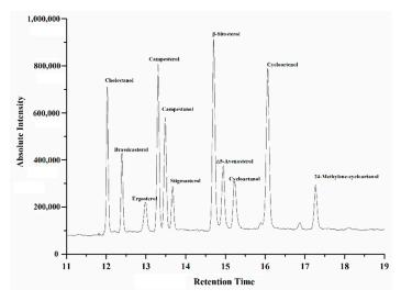
Figure 1. Total ion chromatogram of silylated sterol standards by GC-MS analysis.
