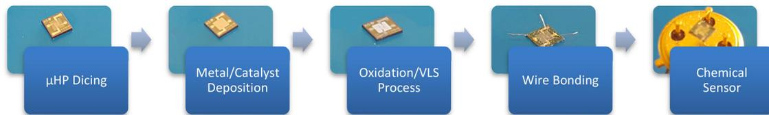
**Figure 2.** Flow-chart of the integration of metal oxide (MOX) nanowires on ams  $\mu$ HPs to fabricate chemical sensors.
