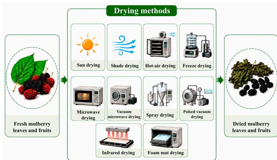
Figure 8. Schematic diagram of the main drying technology routes for MLs and MFs.
