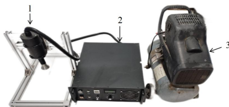
Figure 1. Schematic diagram of the gliding arc discharge low-temperature plasma system; 1—plasma nozzle; 2—plasma power supply; 3—booster pump.
