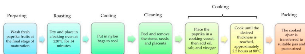
Figure 2. Flowchart of Ajvar production.
