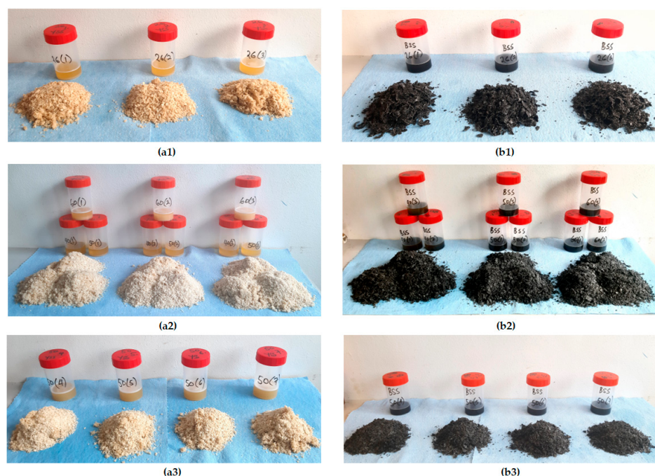
Figure 3. Extracted crude oil with sediments following the factorial design for yellowish sesame (a1–a3) and blackish sesame (b1–b3) for the control temperature of 24 °C (a1,b1) and heating temperatures of 40 °C, 50 °C, and 60 °C (a2,a3,b2,b3) for various heating times of 15, 30, and 45 min.
