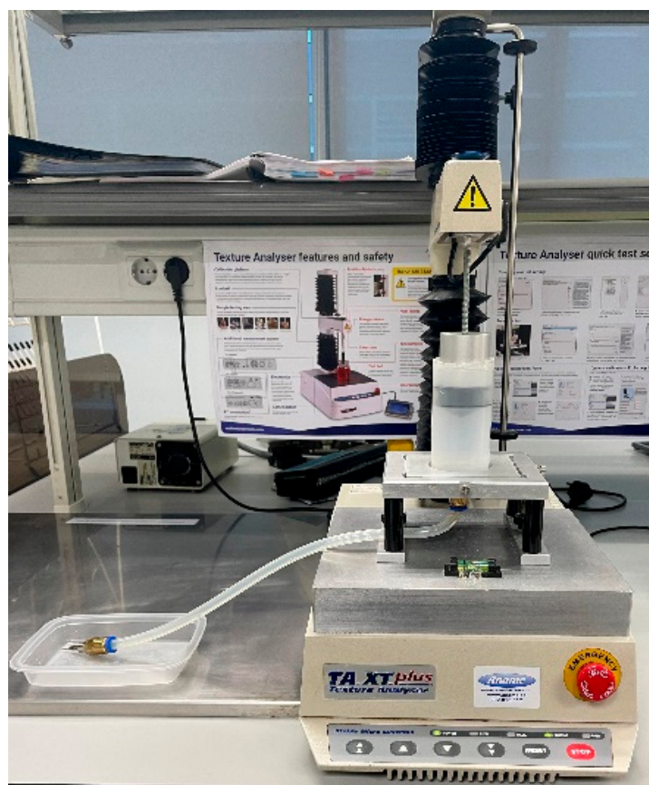
Figure 1. Extrusion test set-up.
