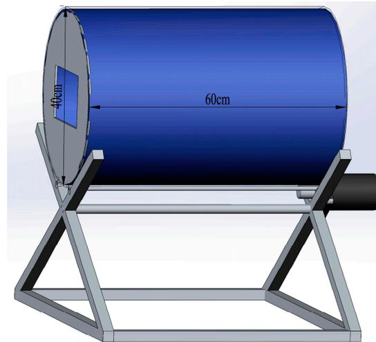
**Figure 1.** The motorized rotating drum used for the physical pretreatment of grapes, lined internally with sandpaper to remove the surface wax.
