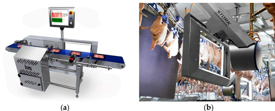
**Figure 4.** The application scenario of machine vision technology in livestock and poultry meat quality detection: (a) quality classification of pork; (b) quality detection of chicken carcass.
