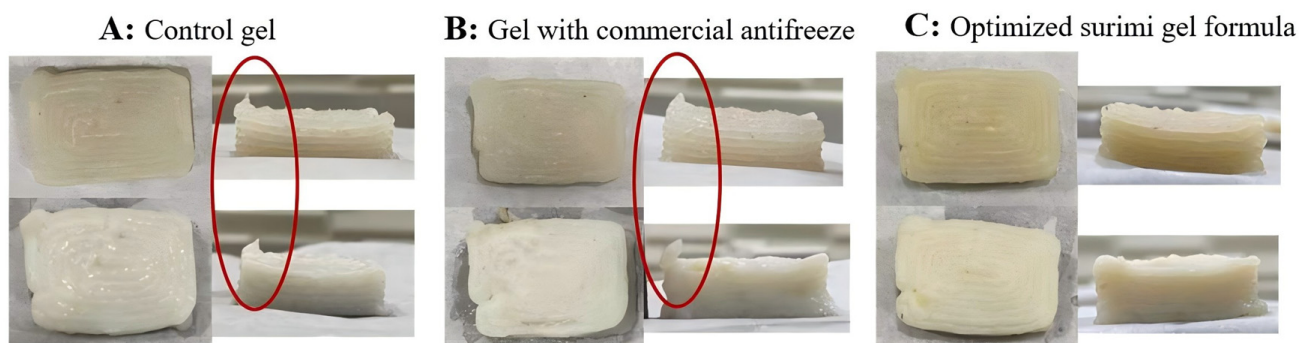
Figure 10. Representative images of 3D printed surimi gels: control group (A); surimi with 8% commercial antifreeze (B) and optimized surimi gel formula (C), with red circles indicating 3D printing defects.
