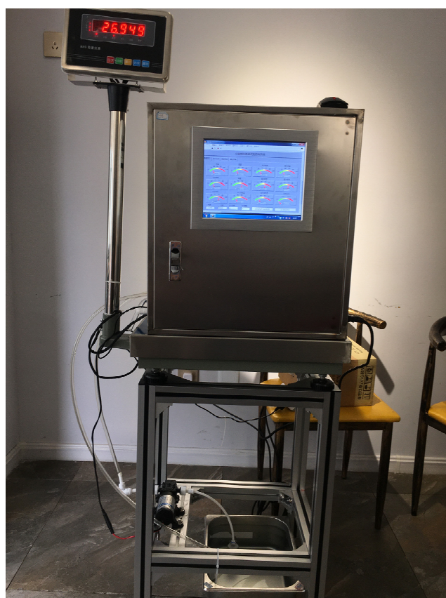
Figure 1. Fixed-bed drying test device of increased efficiency by condensation.
