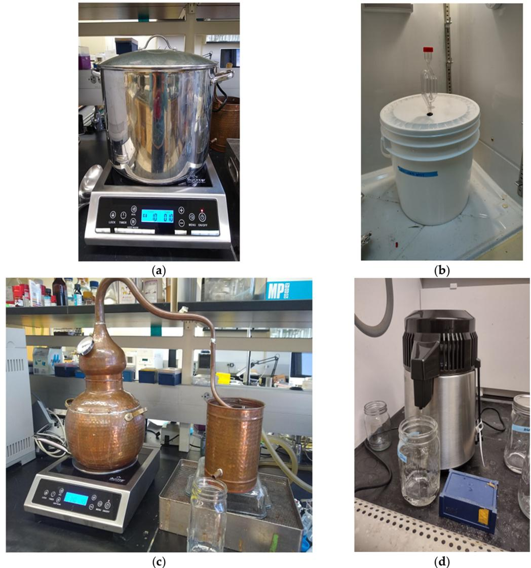
**Figure 4.** Laboratory equipment for new-make bourbon whiskey production: (a) mashing; (b) fermentation; (c) first-pass distillation; (d) second-pass distillation.
