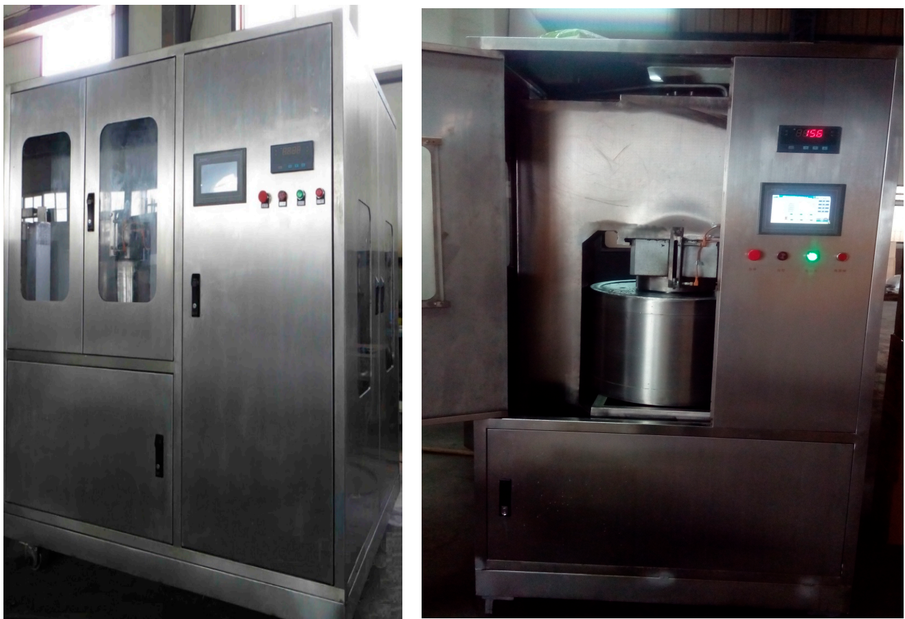
Figure 1. Appearance (left) and internal cavity structure (right) of high-pressure equipment (Bao Tou KeFa, Baotou, China).
