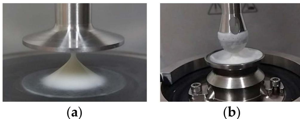
**Figure 1.** Detailed view of (a) the geometry used in rheometry and (b) the configuration used in tribometry.
