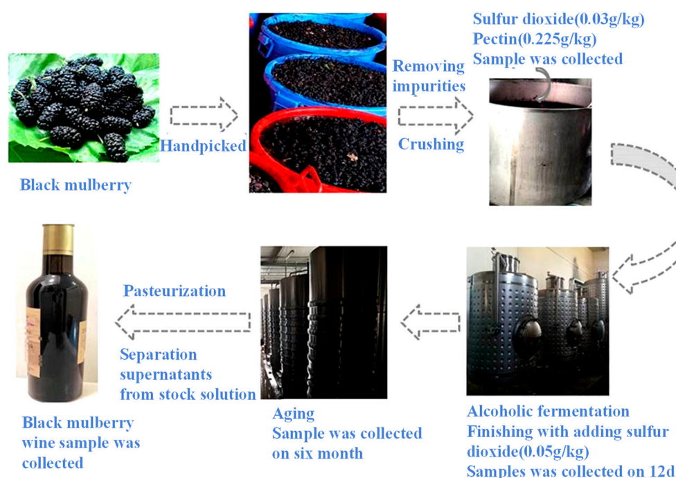
Figure 1. Schematic diagram of mulberry wine fermentation process.
