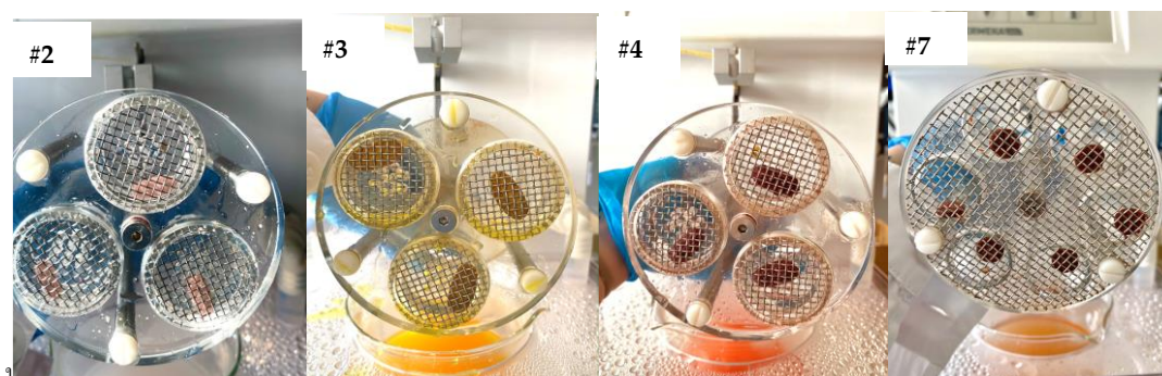
Figure 1. The appearance of the non-compliant tablets after the disintegration test. The test was performed using water at 37 °C as the immersion liquid. For samples #2, #3, and #4 (film-coated tablets), the disintegration time was set at 30 min, while for sample #7 (uncoated tablet) the time was set at 15 min. Apparatus B was used for samples #2, #3, and #4 (diameter > 18 mm) and apparatus A was used for sample #7 (diameter < 18 mm). Disks have been used for all the samples.
