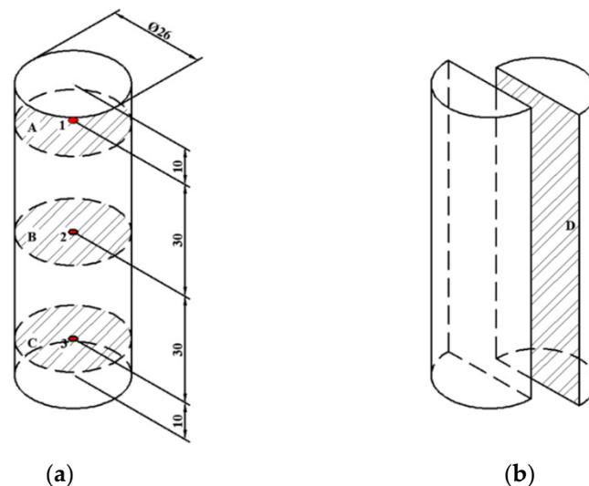
**Figure 3.** The location of fiber optic sensors (1, 2, 3) and four layers (upper, A; middle, B; lower, C; longitudinal, D) in the beef sausage sample for temperature distribution measurement (all measured in millimeters). (a) Detailed diagram of sample. (b) Longitudinal section of sample.
