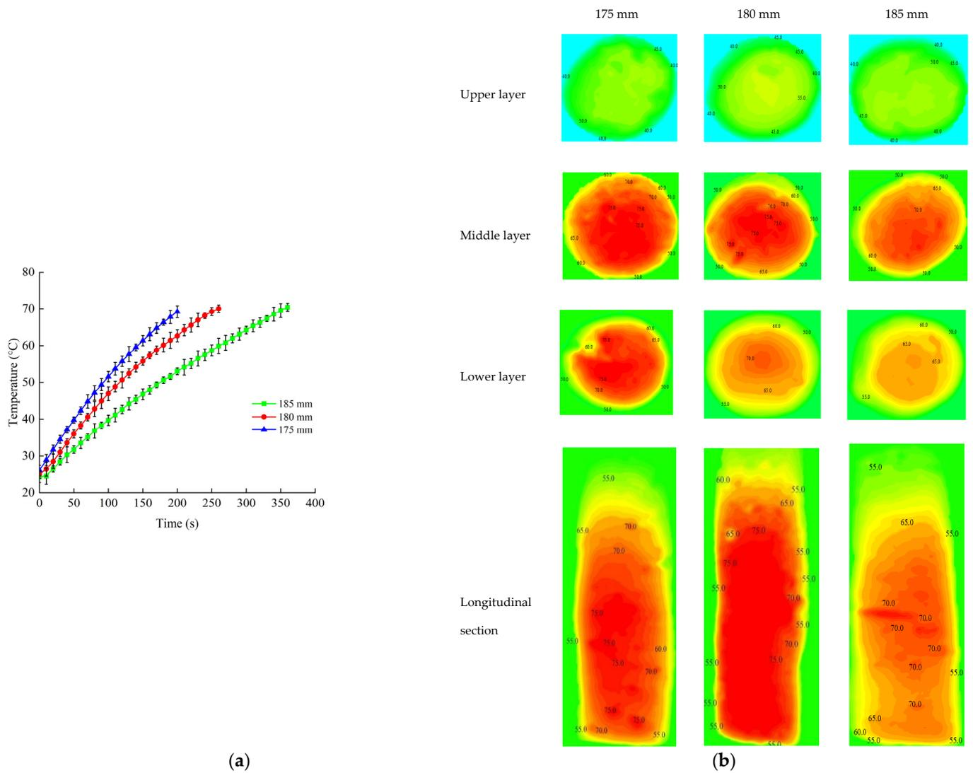
**Figure 6.** Time–temperature heating curves of beef sausages (a) and the contour plots of temperature distribution (b) at different electrode gaps (175, 180 and 185 mm) at a sample height of 80 mm and when the temperature was initialized at 25 °C.
