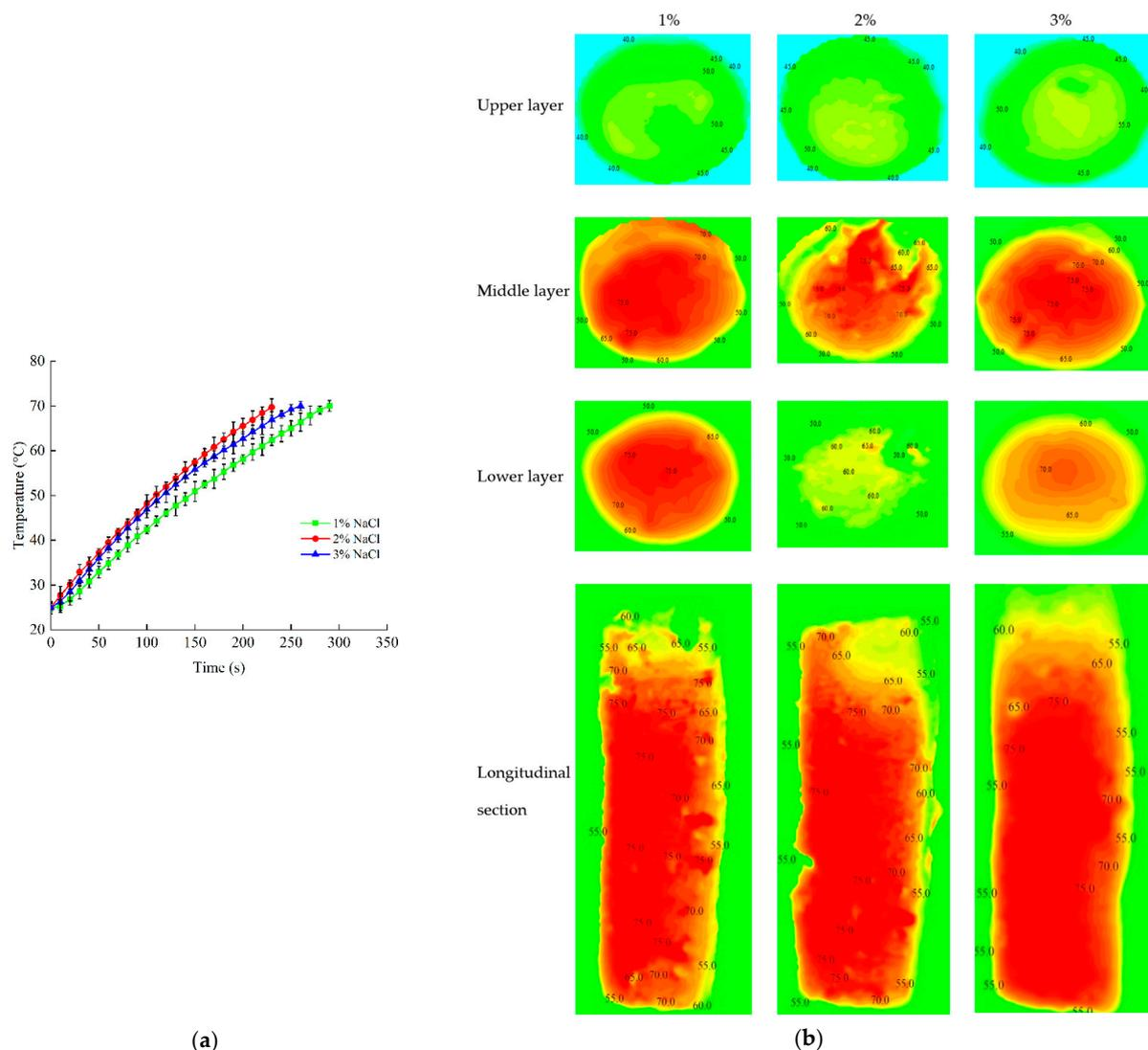
**Figure 8.** Time–temperature heating curves of samples (a) and the contour plots of temperature distribution (b) with different NaCl contents (1%, 2% and 3%) at an electrode gap of 180 mm, a sample height of 80 mm and when the temperature was initialized at 25 °C.
