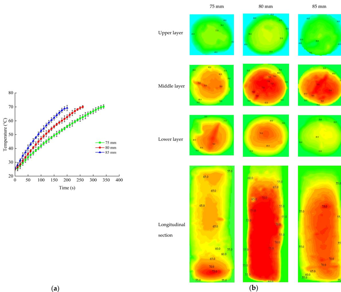
**Figure 7.** Time–temperature heating curves of beef sausages (a) and the contour plots of temperature distribution (b) at different sample heights (75, 80 and 85 mm) under an electrode gap of 180 mm and when the temperature was initialized at 25 °C.
