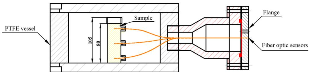
**Figure 2.** Detailed cross-section view of the sterilization kettle with beef sausage placed in the center and fiber optic sensor inserted in the sample.
