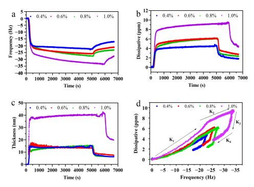
**Figure 4.** The frequency (**a**), dissipative (**b**) and thickness (**c**) during the adhesion and washing at the MCT-coated sensors; D-f plots (**d**) during adhesion and washing processes ( $K_1$ ,  $K_2$ ,  $K_3$ , and  $K_4$  were the slopes at four different phases, respectively).
