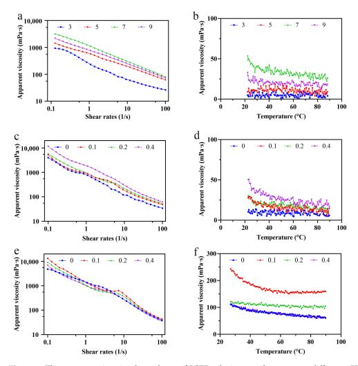
**Figure 3.** The apparent viscosity dependence of LSEP solutions on shear rates at different pH (a), CaCl<sub>2</sub> concentration (c), and NaCl concentration (e); the apparent viscosity dependence of LSEP solutions on temperature at different pH (b), CaCl<sub>2</sub> concentration (d), and NaCl concentration (f).
