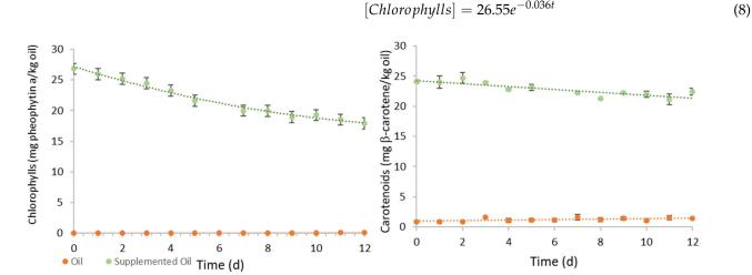
**Figure 6.** Evolution of the contents of chlorophyll pigments (mg pheophytin a/kg oil) and carotenoids (mg β-carotene/kg oil) in non-supplemented and supplemented oil samples, along storage at 60  $^{\circ}$ C for 12 days under dark.
