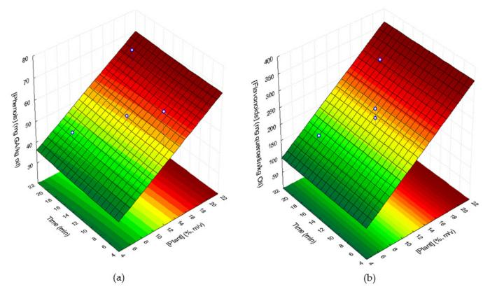
**Figure 4.** Response surfaces describing the contents of phenolic compounds, expressed in mg gallic acid (GA) equivalent/kg of oil (a) and flavonoids, expressed in mg quercetin/kg oil (b) of supplemented sunflower oil with lyophilized *C. maritimum* extracts, as a function of lyophilized *C. maritimum* concentration and UAE time.
