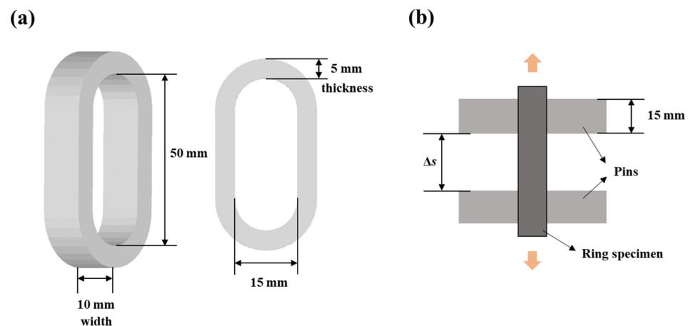
**Figure 1.** Dimensions of the ring specimen (a) and a schematic drawing of the front view of the ring tensile test (b).
