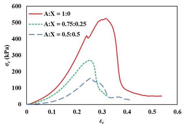
**Figure 2.** Representative stress-strain curves obtained by compression test for agarose-xanthan gel systems. A is agarose and X is xanthan.
