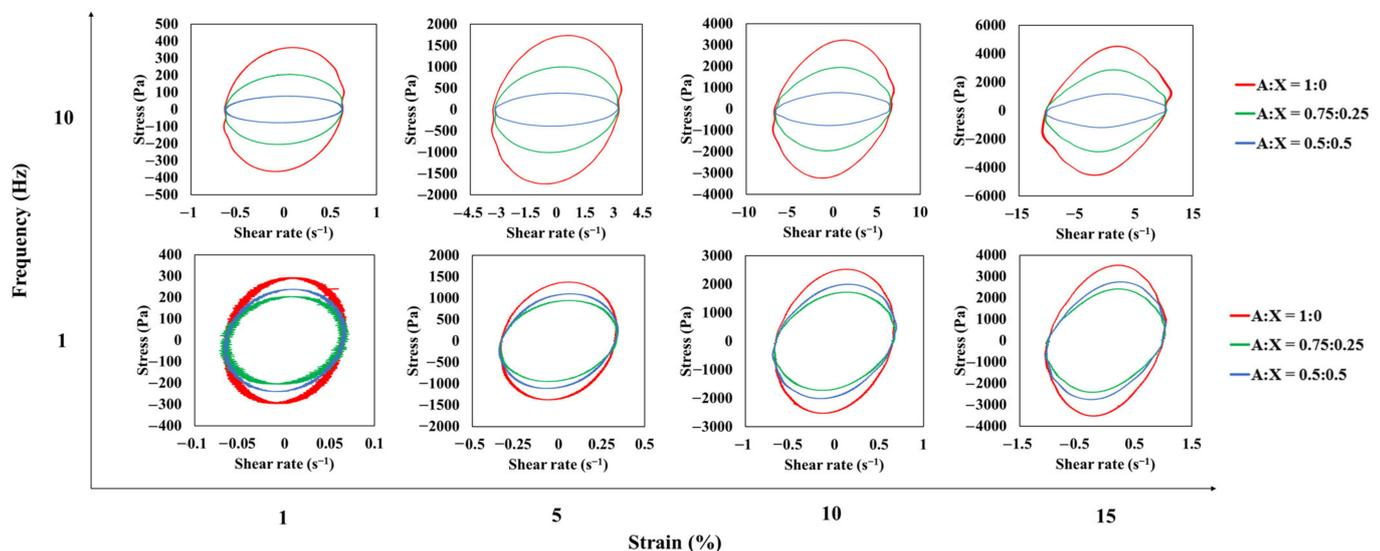
**Figure 7.** Viscous Lissajous-Bowditch curves for agarose-xanthan gel systems measured at different strains and frequencies.
