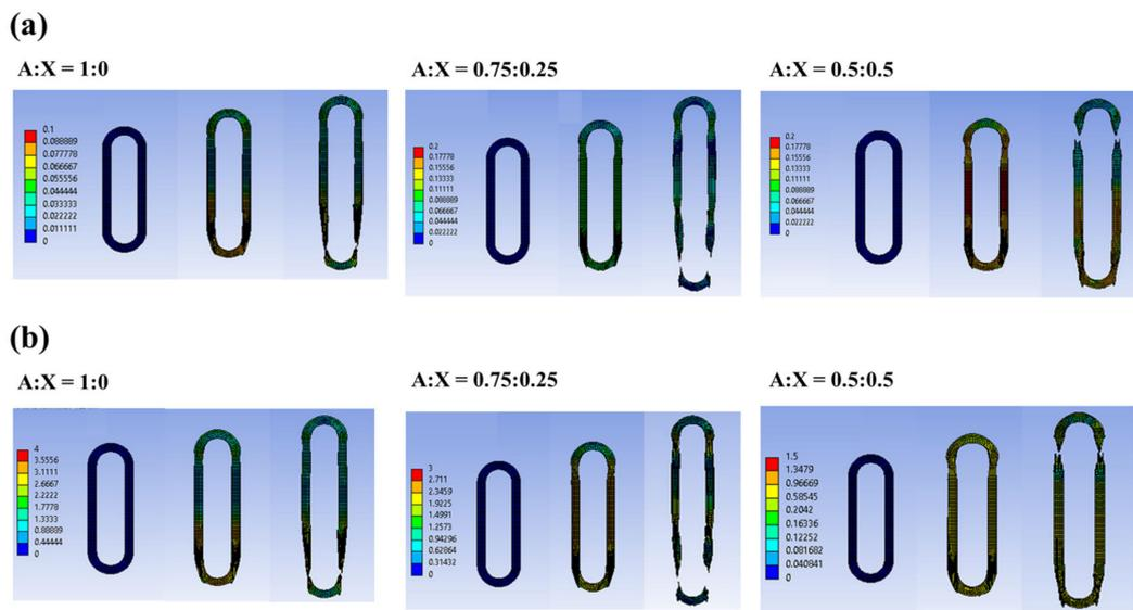
**Figure 5.** Simulation results of sample elongation and failure examined by a ring tensile test. (a) strain distribution, and (b) stress distribution in the sample during ring tensile measurement. A is agarose and X is xanthan.
