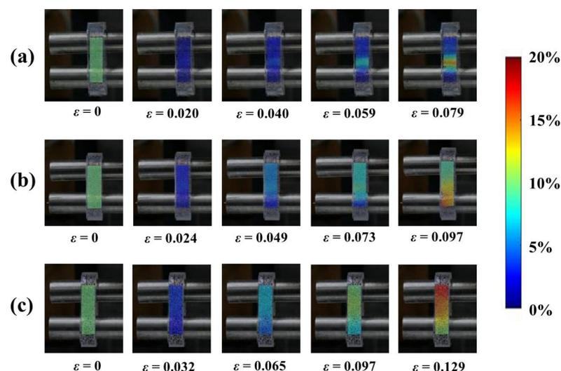
**Figure 4.** Digital image correlation (DIC) analysis of the local strain of agarose-xanthan gel systems during a ring tensile elongation until failure: (a) A:X = 1:0; (b) A:X = 0.75:0.25; (c) A:X = 0.5:0.5. A is agarose and X is xanthan.
