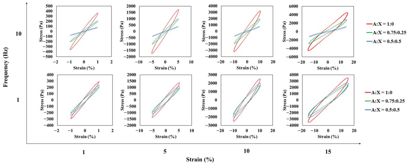
**Figure 6.** Elastic Lissajous-Bowditch curves for agarose-xanthan gel systems measured at different strains and frequencies.
