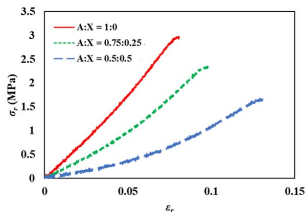
**Figure 3.** Stress-strain curves obtained by ring tensile test for agarose-xanthan gel systems. A is agarose and X is xanthan.
