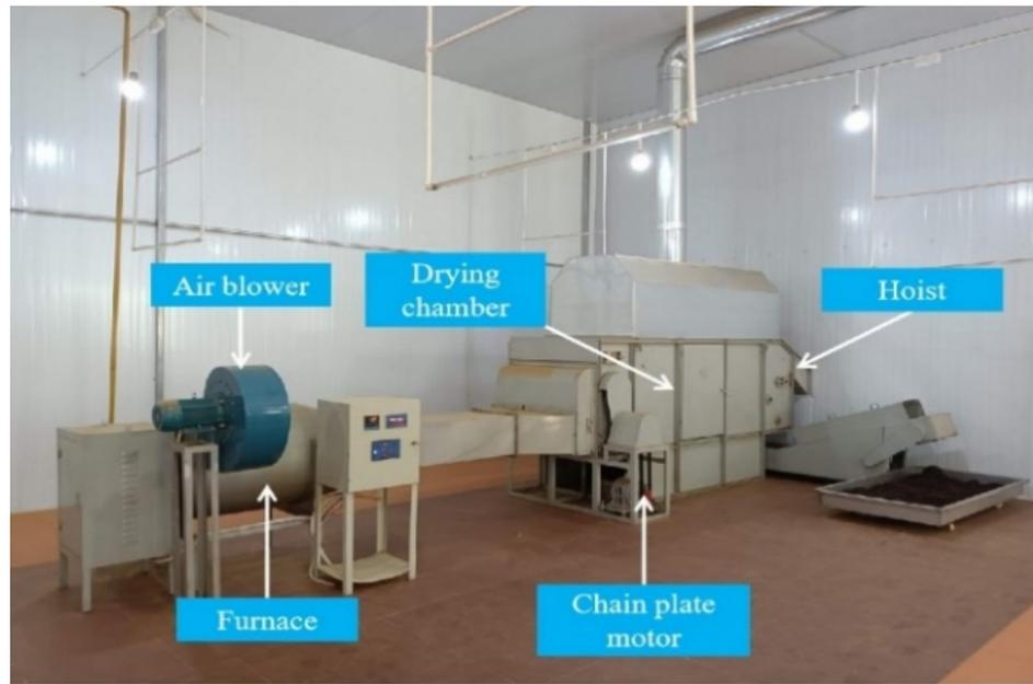
Figure 2. Photograph of the gas-type industrial drying system of black tea.
