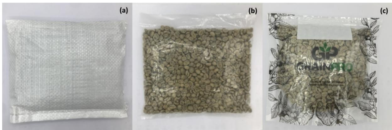
**Figure 1.** Packages for GCB storage (a) plastic woven bag (PW), (b) low-density polyethylene bag (LDPE) and (c) GrainPro® (GP).
