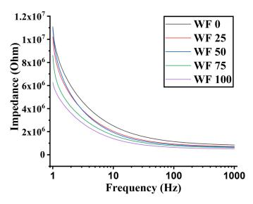
Figure 8. Graphs representing impedance of various samples.
