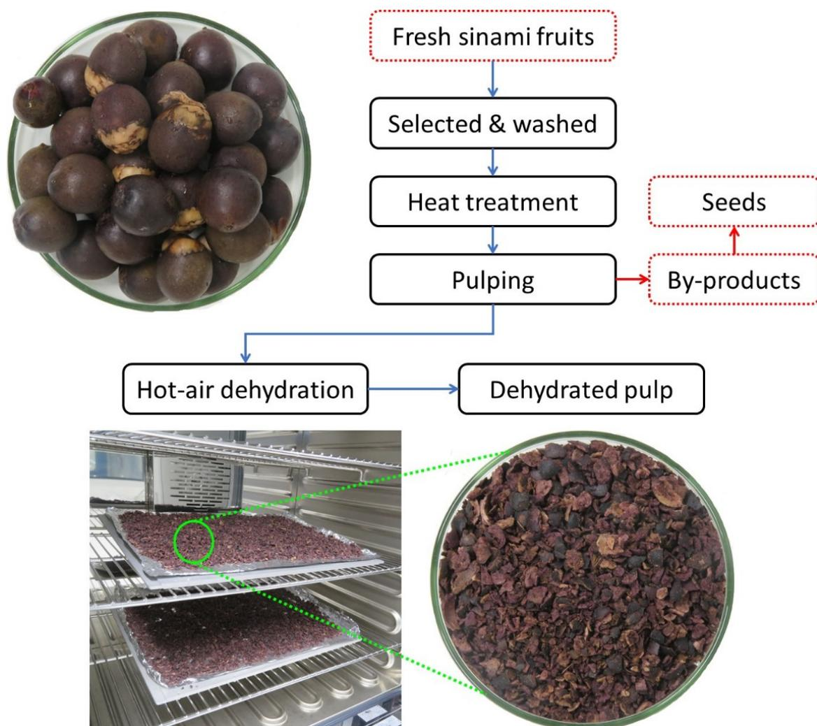
**Figure 1.** Flowchart of the process for obtaining dehydrated pulp from sinami fruit.
