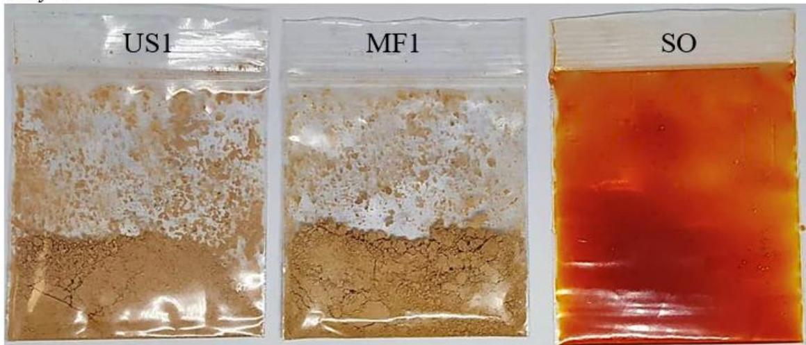
**Figure 5.** Images of SO, US1 and MF1 samples packed in zip lock bags at day 0 and day 30 of storage at room temperature (28–30 °C). SO, shrimp oil; US1, ultrasonicated KBPI-KC-SO microcapsules containing 0.1% SO; MF1, microfluidized KBPI-KC-SO microcapsules containing 0.1% SO.
