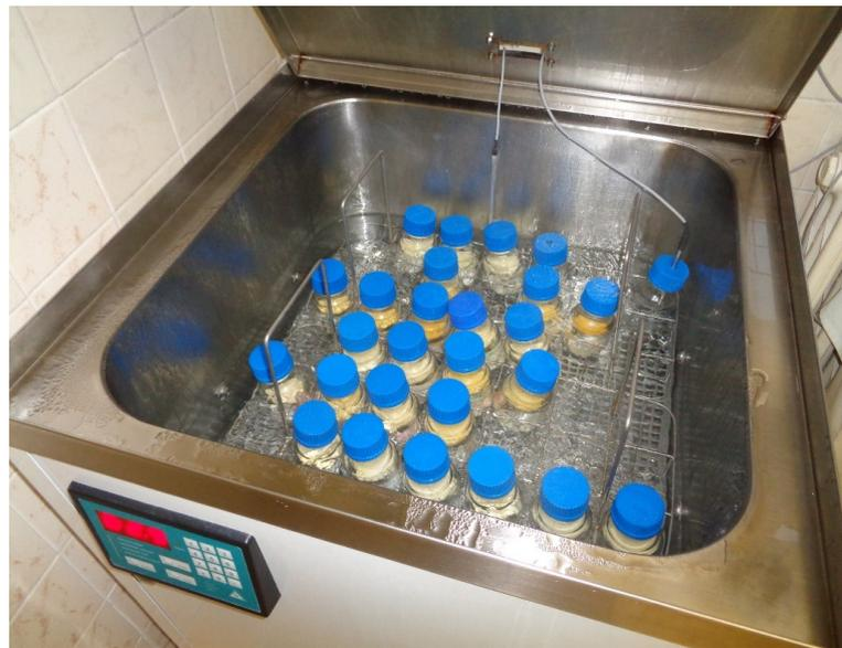
**Figure 1.** Bottles with collected milk in the warming section of the pasteurization device. The temperature is monitored and recorded inside the water bath and in the bottle containing the milk analog.
