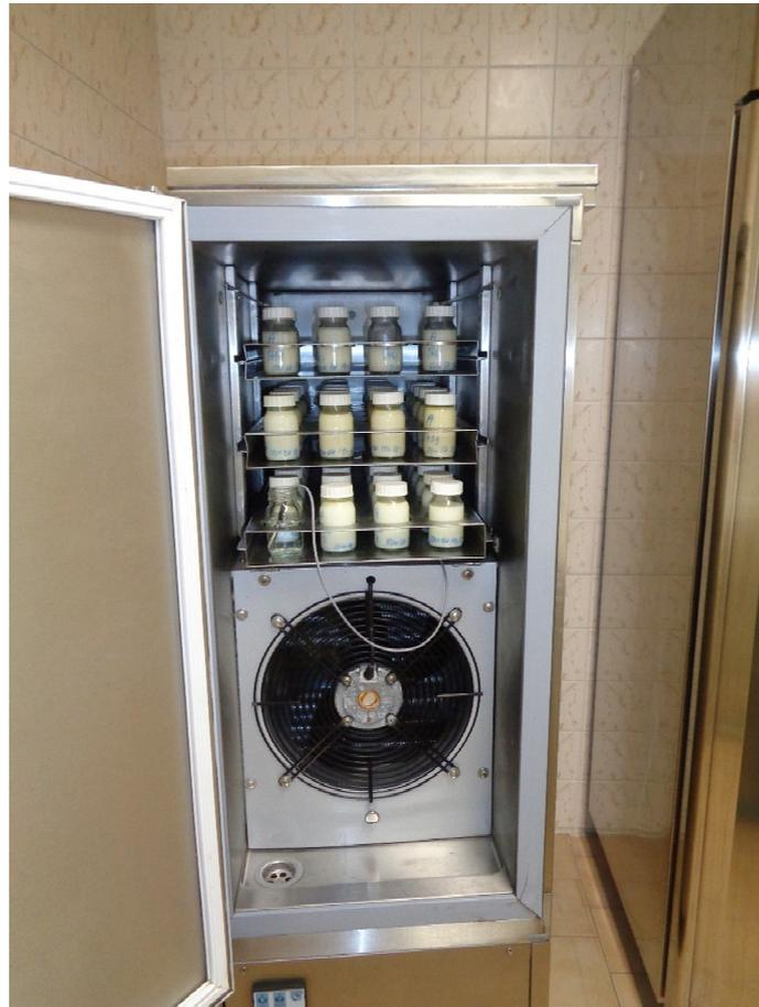
**Figure 3.** Distribution bottles in the blast freezer. The temperature of the air and inside the bottle containing the milk analog is recorded.
