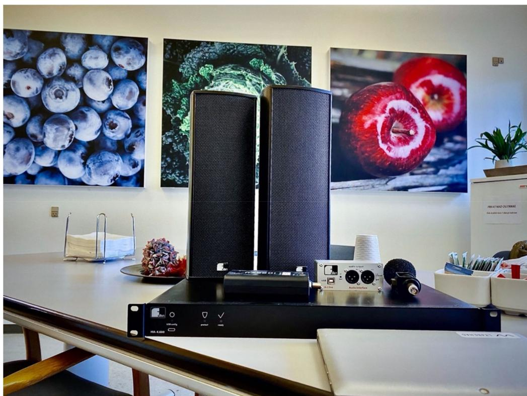
**Figure 2.** Acoustic and audio equipment. Panels: AKUART On the Wall 60 wall absorbers. Audio equipment: Fohhn Audio Scale-1 speakers; Fohhn Audio MA-4.100 amplifier; Fohhn Audio A1-Live USB-sound card, and MacBook Pro laptop.
