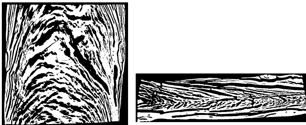
Figure 9. Microstructure of freeze-dried SPI extrudate, obtained with X-ray measurements. Sample was extruded at 50% ( w/w ) moisture content and material temperature of 124 °C before entering the cooling die. Top view ( left ) and side view ( right ) are displayed. Flow direction is directed from bottom to top for the top view and left to right for the side view.
