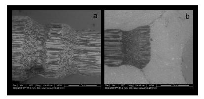
**Figure 9.** BE LV-SEM image of a debonded ARL post, (**a**) with sheared off retentive elements and (**b**) attached to the core material structure (a:  $40\times$ , bar = 1 mm, b:  $140\times$ , bar =  $300 \text{ }\mu\text{m}$ ).
