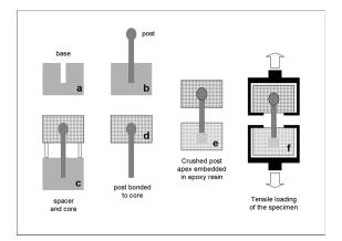
Figure 2. The specimen preparation procedure employed.
