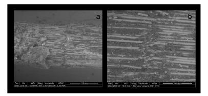
**Figure 8.** BE LV-SEM image of a fractured PRW post, (**a**) with details of the sheared off spherical protrusions (**b**) and the cut fibers at the contact of the protrusions with the main body (a:  $40\times$ , bar = 1 mm, b:  $140\times$ , bar = 300 µm).
