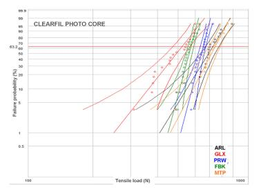
Figure 4. Weibull plot for the posts restored with CPC.
