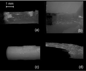
**Figure 7.** Stereomicroscopic images of fractured posts and core build-up materials (25×, bar = 1 mm). (a) FBK coronal part with broken serrations; (b) FBK broken part into the core material; (c) PRW with sheared off spherical retentive elements; (d) ARL body fracture.
