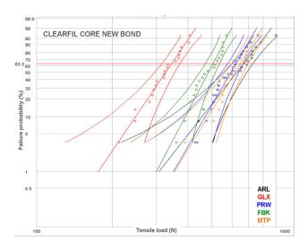
Figure 6. Weibull plot for the posts restored with CNB.
