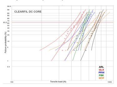
Figure 5. Weibull plot for the posts restored with CDC.
