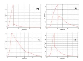
**Figure 3.** Load–displacement curves of ARL (**a**), FBK (**b**), GLX (**c**) and MTP (**d**). Note the stepwise loading in FBK after initial fracture.
