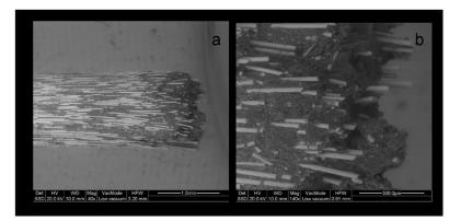
**Figure 10.** BE LV-SEM image of a fractured MTL post, (**a**) with details (**b**) of non-uniformly distributed fibers (a:  $40\times$ , bar = 1 mm, b:  $140\times$ , bar = 300 µm).
