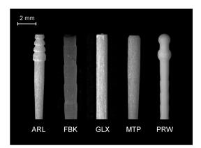
**Figure 1.** Stereomicroscopic image of the coronal and middle body parts of the posts used in the study (10×, bar = 2 mm).
