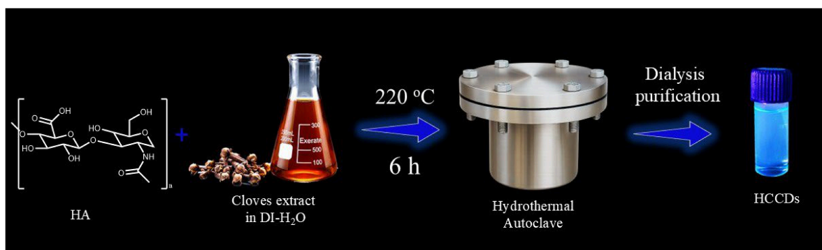
Scheme 1. Schematic representation of the hydrothermal synthesis of HCCDs.
