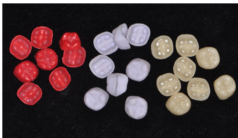
Figure 3. Lithium disilicate wax patterns, cores and veneered crowns.
