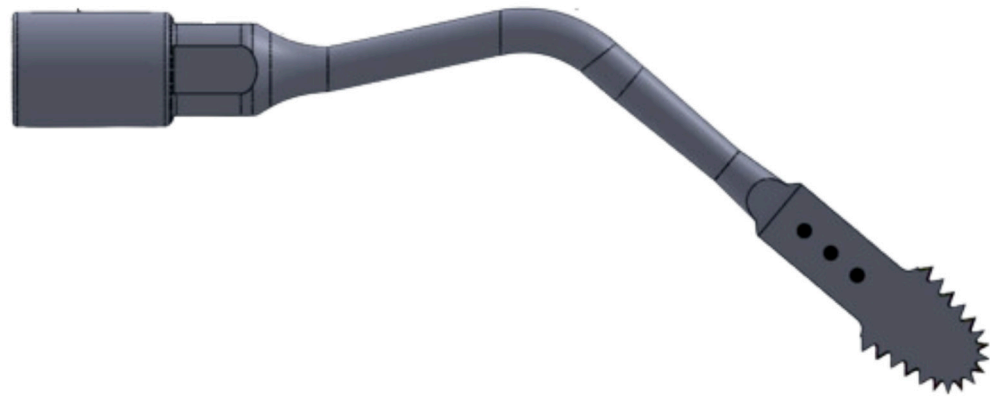
Figure 2. Piezoelectric Saw—13 mm active length, with a width ranging from 3.3 mm to a thickness of 0.35 mm. (Source: Author 2024).
