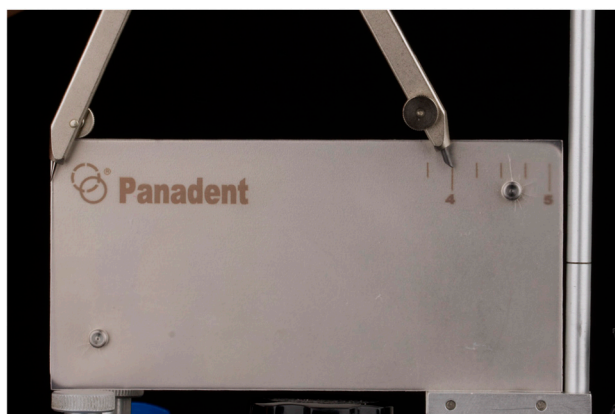
Figure 4. Selecting the 4-inch radius on the Broadrick flag with the compass.
