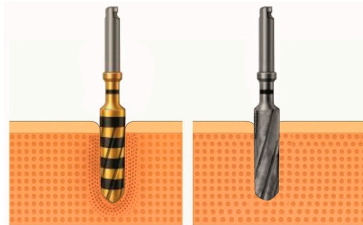
Figure 1. Comparison between a densification drill (Densah®) and a conventional helical drill (left and right images, respectively), showing the radial compaction of bone particles characteristic of bone densification.
