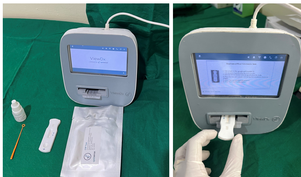
Figure 1. Armamentarium used for study: saliva collection kit (sample collection loop and buffer solution) and CRP test kit along with VIEWDx analyzer.
