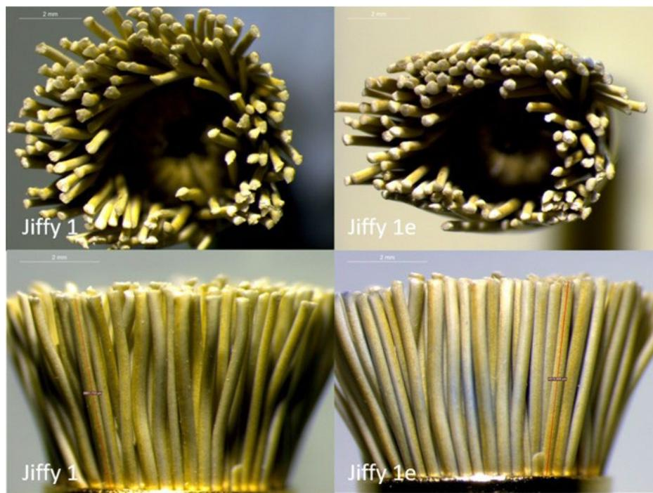
**Figure 13.** Representative optical microscope images (1.6 $\times$ ) of JPB after the first (1) and after the fifth application (1e). A gradual fusion of the bristles, a decrease in the tool's diameter, and rounding of the bristle tops was observed.
